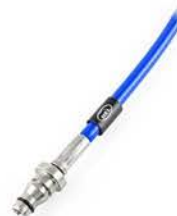
HEL flexible braided clutch line for Ford Focus MK3 RS and ST right hand drive (2013-2018) Part No. CCK157
